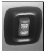
With the ignition on, press and release the rear of the switch and the glass panel will open to the vent position. Open the sunshade by hand when using the vent position.
